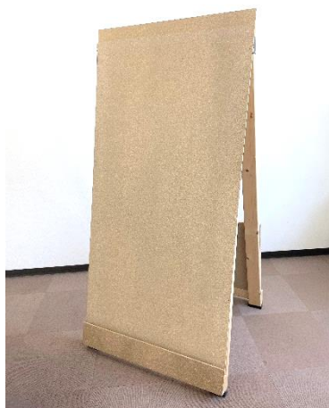
Wooden board made from recycled wood waste as raw material and used for housing
