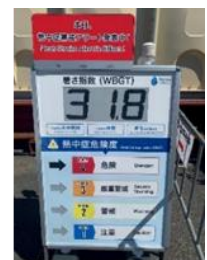
Display board showing the heat stress index installed at the entrance of a venue
