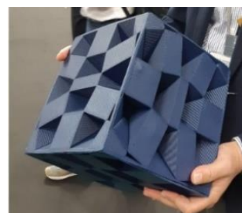
Podium parts fabricated with a 3D printer using recycled plastic
