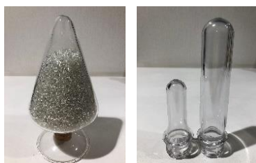
Resin (left) and preform (right) manufactured through the bottle-to-bottle recycling process
